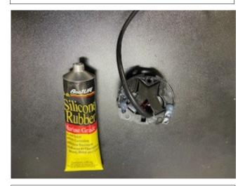
On the bottom side of the 2279815 light assembly put a spot of silicon on either side of the rear of the light.
