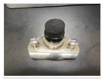
Apply the spacer foam to the top of the light base. Once the cover is placed on the light assembly, the spacer will help apply downward pressure to the light base while the silicone is setting up. Technically, it is not needed once the silicone sets up, but it will not harm anything long term. It can be left in place.
