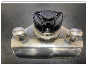
Connect the wires to the power leads coming up through the chock base. Insert the #6 pan head screw in the forward hole in the light assembly. You will tighten it down into the hole you drilled in the nylon screw.
