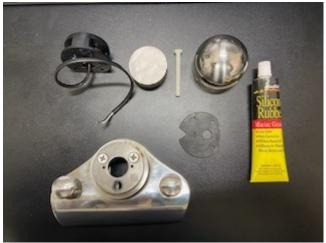
Shown above (with the exception of an 1/8" drill bit and drill) are all of the necessary components to do the LED light base conversion on your Boston Whaler 1748820 bow light/chock assembly. You will need to order a 2273864 nav light cover, a 2279815 bow light, and a CONV-1748820 kit. The kit includes a 1/4-20 nylon machine screw, one #6 pan head self tapping screw, and an adhesive backed foam spacer.
