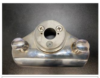
Using an 1/8" drill bit carefully drill in the center of the nylon bolt. It needs to be deep enough to accommodate the #6 pan head screw.
