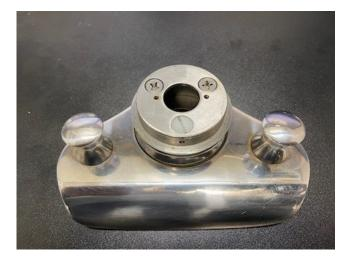
Once the stainless steel cover and the old light base have been removed you will have access to the 3 1/4-20 machine screws that secure the chock base to the hull of the boat. Remove the forward-most machine screw and replace with the nylon screw. Make sure to apply silicone to the threads of the screw before inserting. Carefully screw it in place until it is fairly tight.
